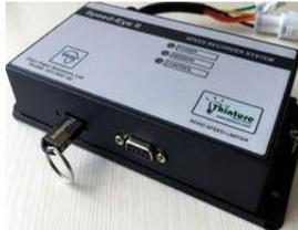
Speed recorder & limiter is an advanced form of normal speed limiter device. Apart from speed limiting function, this device can act as a data logger also. Our speed recorder, Speed-eye II can record highest speed value, real time for every minute and record for more than 5 days. This data can be retrieved any time using a simple USB flash disk.
